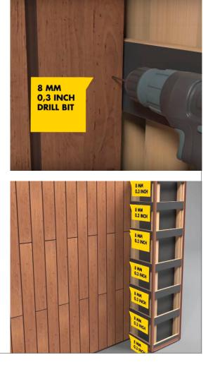
• Fix the cladding with SFS Intec HPL Fast Fixing Screws.
